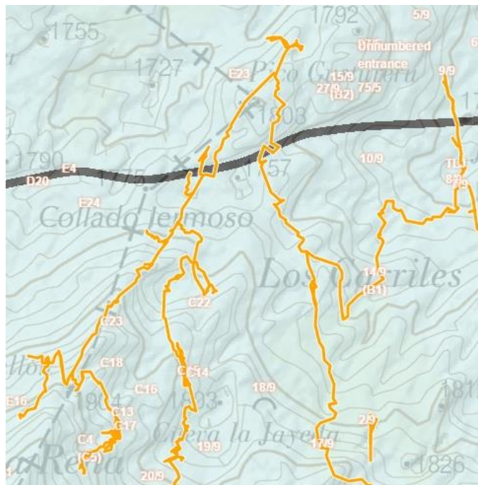
Plate 22 – Overlaying the survey data onto topographical and geological maps reveal a fault (thick black line) crossing at the location of the downstream sump climb ('kink' in Underground Overdrive ). From maps created by Martin Laverty (OUCC)
